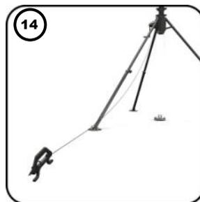
Take one **NORMAL** step for each meter of height of the mast. 15 Meters = 15 Steps
