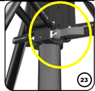
Slowly release the cam lock and allow the first mast pole to rest on the lift base plate.
