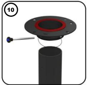
Add the red primary guy ring and pin it to the bottom hole on the mounting pole.
