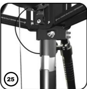
Raise the mast pole until the castle cuts on both mast poles nest together.
