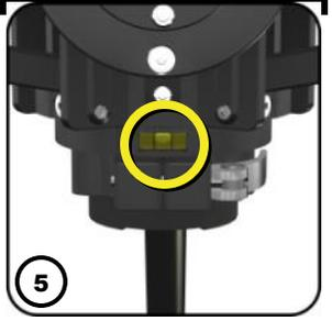
Level the tripod by using the three bubbles levels.
