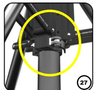
Lock the cam lock and lower the lift base plate to the ground. Insert another mast pole.
