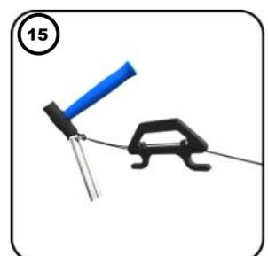
Stop - unwind the remaining guy rope and drive a stake into the ground. Clip Guy rope to stake
