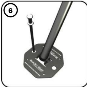
Secure the tripod by driving stakes through the two holes on each of the tripod base plates.
