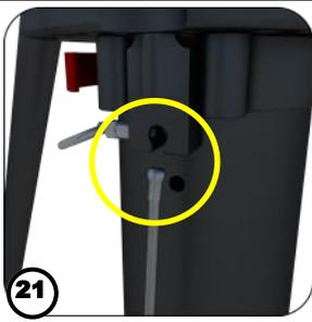
Release the ball stop from the holder and wind up the cable on the winch.
