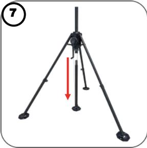
7 Release the cam lock and SLOWLY lower the mast to the ground. Remove the mast pole.
