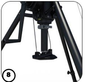
8 Raise the lift base plate until it nests firmly into the next mast pole.
