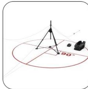
Attach the winch handle. Pay out the cable by turning the winch handle counter clockwise
