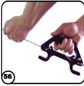
Lock the primary guy ropes by pulling a small amount of slack in. Use your finger and loop the guy rope over the front lip of the guy handle. Pull the guy handle towards the mast to remove any slack in the rope.
