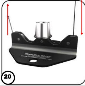
20 Pay out enough cable to go through the pulleys and back up to the ball stop holder.
