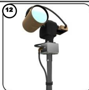
Attach and secure your devices to the mast. Use velcro straps to secure any cables.
