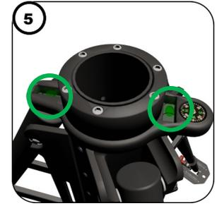
Level the tripod by using the two bubble levels and adjusting the tripod legs.
