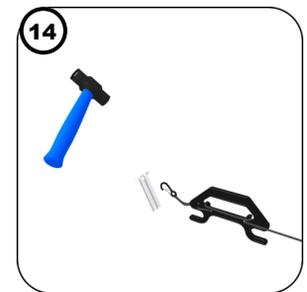
Drive a stake into the ground at an angle and attach the guy rope.
