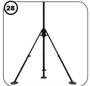
Insert the base pole, slowly lower it to the ground and lock the cam lock.
