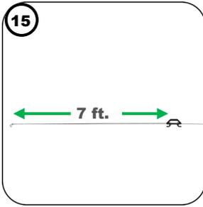
Slide the handle towards the mast approx. 7 feet. This will take up the slack in the guy rope during deployment and prepare you for incremental guying. Repeat this process until all 4 guy ropes are 90 degrees apart.
