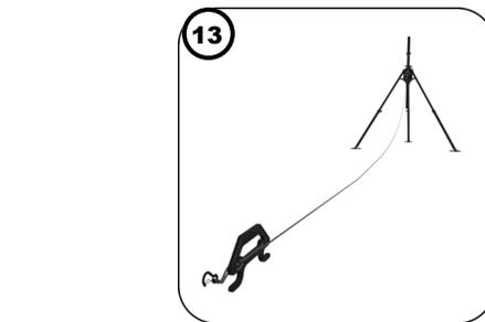
Start at the center of the tripod and unwind the guy rope while walking away from the mast. Take one **NORMAL** step for each meter of height of the mast. 15M = 15 Steps. One person should deploy all 4 guy ropes.
