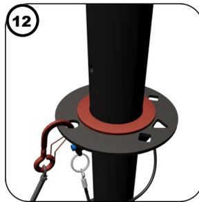
Attach the 1st primary guy rope to the round hole on the red primary guy ring.
